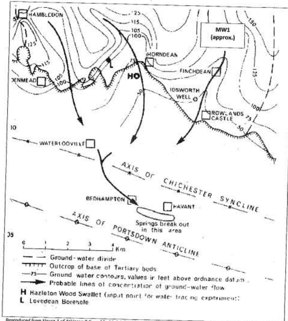
Reproduced from Figure 1 of Atkinson T.C. and Smith D.J. *Rapid Groundwater Flow in the Chalk: an example from South Hampshire*. *G. J. of Eng. Geol.* 1974 Vol 7. Pp 197-205. Contour levels refer to the height of groundwater above ordnance datum, and are not topographical contours.
